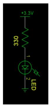
The long lead on the LED goes to Vcc (via the resistor) the short one to ground.
